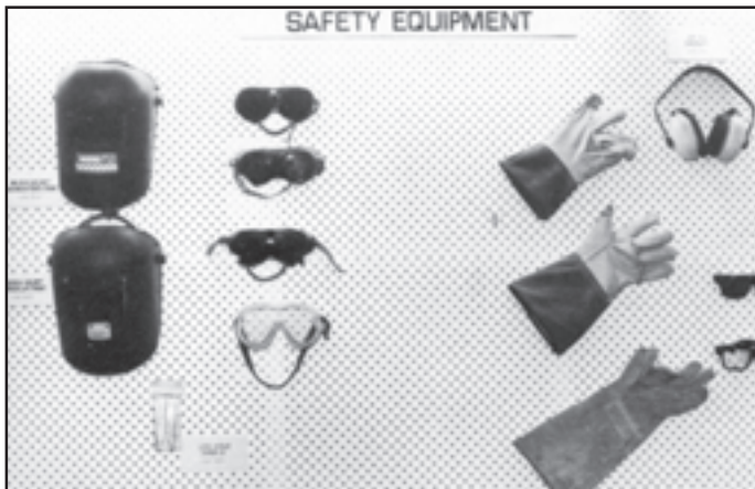
Fig. 8 Typical safety equipment for the protection of eyes, ears, and hands. These are suitable for various tasks, but it is important to select the correct equipment for the work undertaken.
