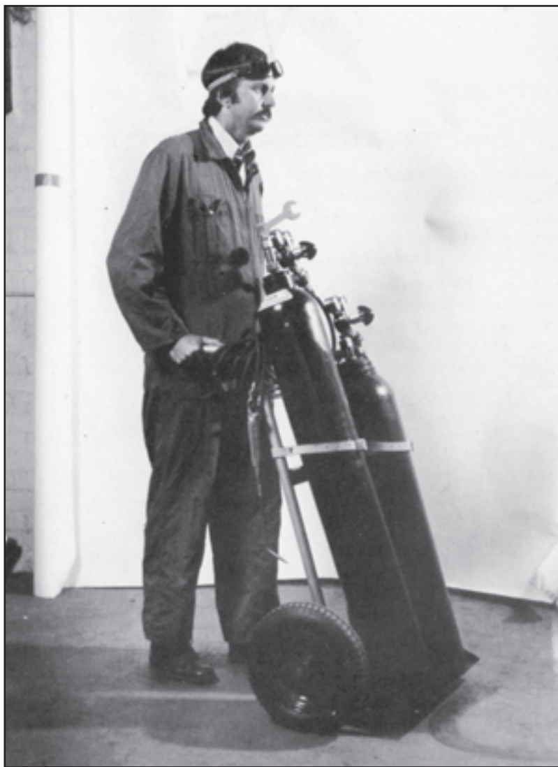
Fig. 1 A typical portable gas plant, with the cylinders securely mounted on a robust, rubber-tired trolley for easy movement. A flashback arrestor is fitted to each regulator. The welder is wearing suitable goggles, overalls and safety shoes. The cylinder key is left fitted to the oxygen cylinder.
