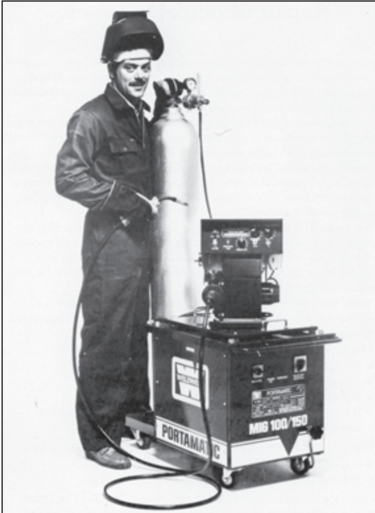
Fig. 6 A MIG (Metal Inert Gas) welding plant. The complexity of this equipment makes it suitable for use only by experienced workers.
